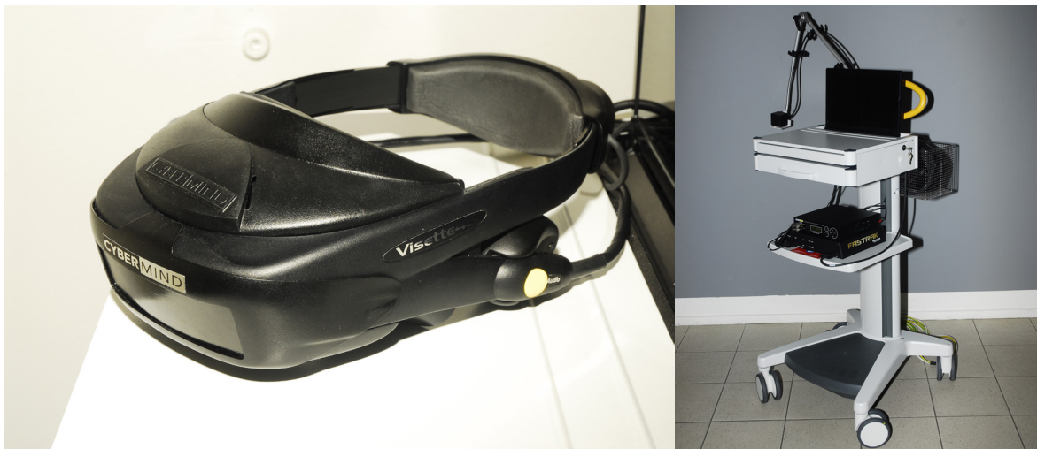
Figure 1.4 | Two main components of the old VR system. Left the visette45 and on the right the Pro Cart
