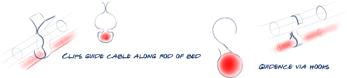
Figure 3.7 | Ideas for guiding the cable along the hospital bed
